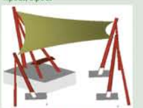
typical concrete foundations pads under mast struts with "duckbill" or similar anchor under guys/tension poles
